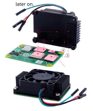
Place the thermal pads from inside the Heatsink pack onto the CPU of the Compute Module 4 board, as shown.
