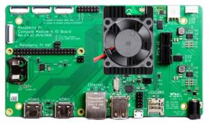
Once the heatsink is in place on the Compute Module 4, gently press it into place on the Base Board, ensuring the connectors (which are off-centre) line up perfectly. You may not hear a click, but you will feel it slot into place.
