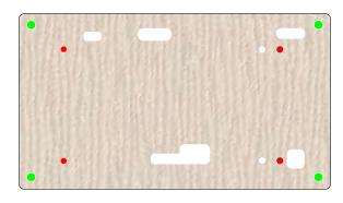
Push the four M2.5 screws up through the four inner holes on the oak base. Using a bit of dexterity, push the four connecting screws (female end) through the outer holes on the oak base, and place the base on a flat surface with the connecting screws and machine screws pointing upwards.
