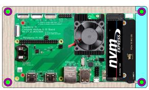
For the last layer, you will find that the female connecting screws have been fully covered, so the washers will have to be placed inline without being "held" in place.... Now drop the **two end plates** into place, ensuring the holes line up with the ports on the circuit board. Finally, place the top cover in place, and use the male connecting screws to hold everything together. It's all good to go!
