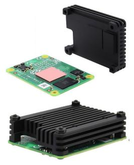
Place the thermal pads from inide the Heatsink pack onto the CPU of the Compute Module 4 board, as shown.
