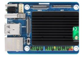
Once the heatsink is in place on the Compute Module 4, gently press it into place on the Base Board, ensuring the connectors (which are off-centre) line up perfectly. You may not hear a click, but you will feel it slot into position.
