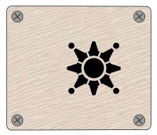
Push the four **M2.5 screws** up through the four inner holes on the oak base, and attach the brass standoffs.
