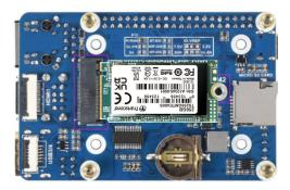
Turn the board over, and remove the brown disc covering the screw hole marked 2242. Align the NVMe drive with the slot and the hole and push the connector into the NVMe drive socket. Use one of the very small screws from the loose bag inside the box to screw the NVMe drive into place with the 2242 hole.
